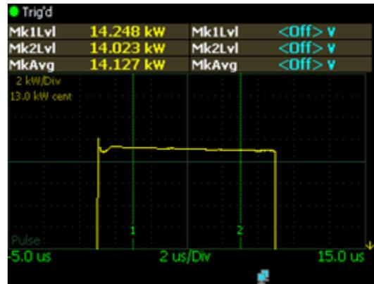
Figure 13 Power at 5 usec pulse width at 1 kHz pulse repetition frequency
