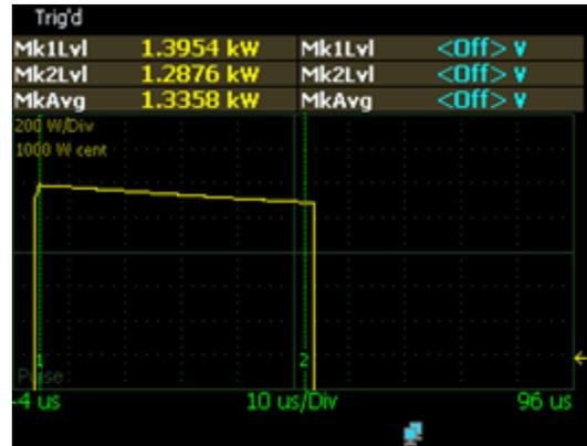
Figure 8 Power at 100 usec pulse width and 1 kHz pulse repetition frequency
