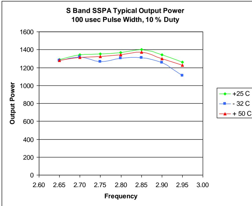
Figure 3 Output power as a function of frequency and temperature.
