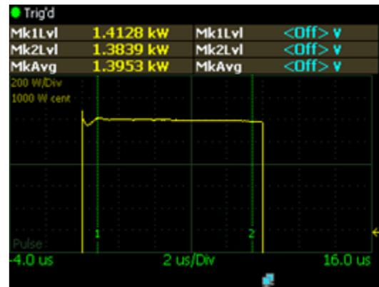
Figure 5 Power at 10 usec pulse width and 1 kHz pulse repetition frequency
