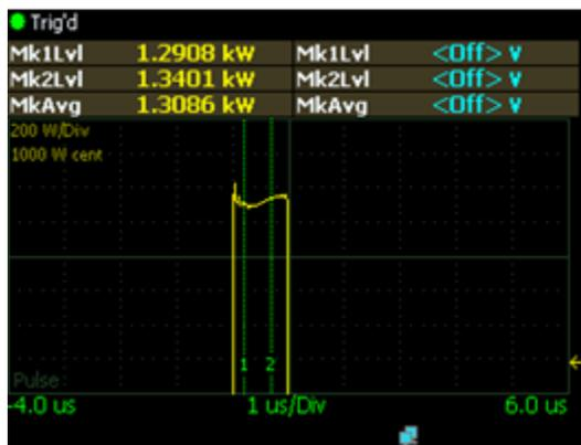
Figure 4 Power at 1 usec pulse width and 1 kHz pulse repetition frequency.
