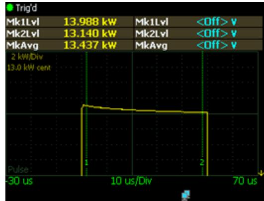
**Figure 15 Power at 20 usec pulse width at 1 kHz pulse repetition frequency**
