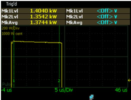
Figure 6 Power at 20 usec pulse width and 1 kHz pulse repetition frequency
