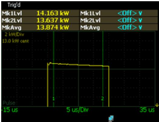
**Figure 14 Power at 10 usec pulse width at 1 kHz pulse repetition frequency**
