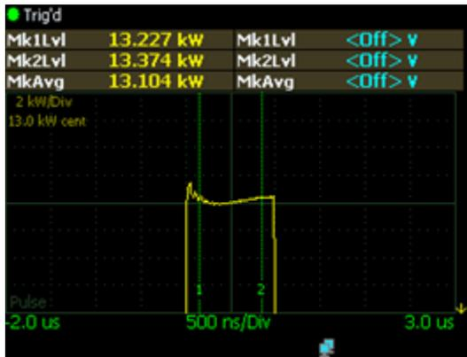
Figure 12 Power at 1 usec pulse width and 1 kHz pulse repetition frequency
