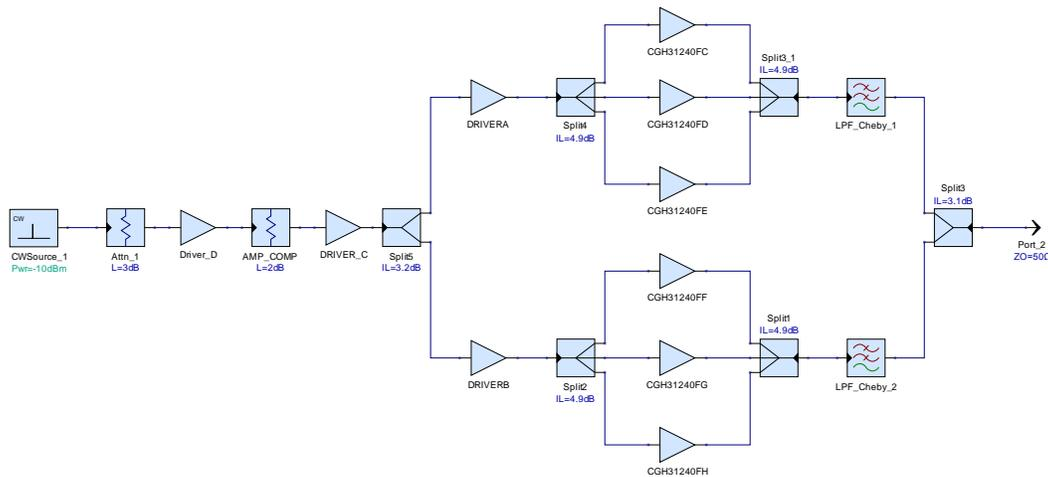
Figure 2 Schematic design of VSS3607 SSPA
