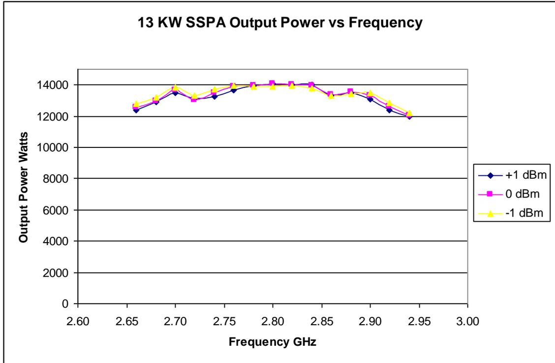
Figure 11 Power as a function of frequency for VSS3605 SSPA
