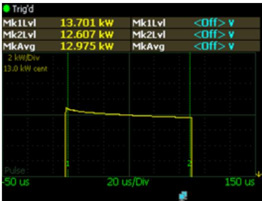
**Figure 15 Power at 100 usec pulse width at 1 kHz pulse repetition frequency**
