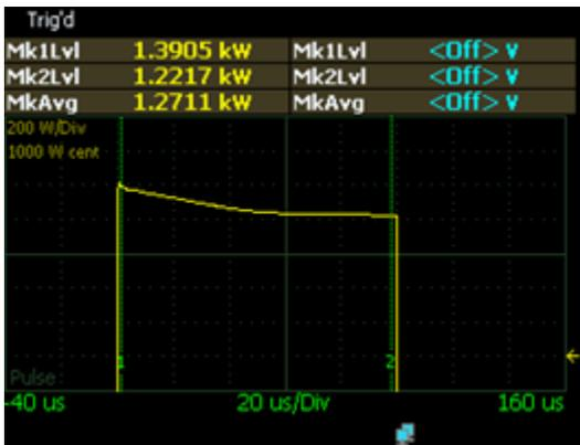
Figure 7 Power at 50 usec pulse width and 1 kHz pulse repetition frequency
